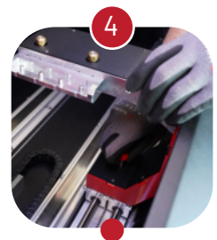
Adjustable product holders adaptable to different lengths and configurations of product
